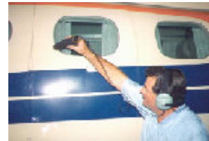
Testing for air leaks with the SG-2sound generator and VPE 1000
