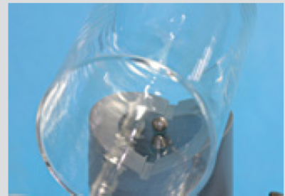
Reference balls with a specially coated finish and dimensional precision to obtain maximum reproducibility of readings.
