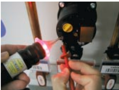
The combination of optical and acoustic readout permits usage in a loud environment.
